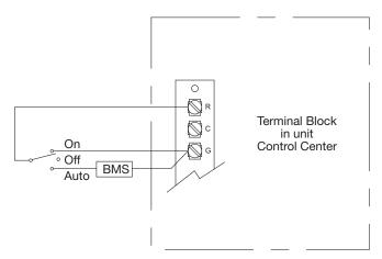
Hand/Off/Auto Switch allows the unit to
